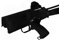
Place Selector Lever in Safe Position
